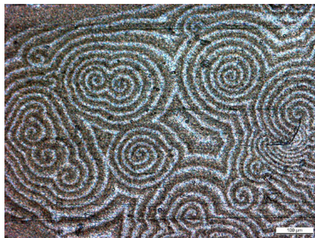
Fig. 4 Optical image of a coating, obtained at current density 1.2 \text{ A dm}^{-2} from the electrolyte B, time of deposition—30 min
